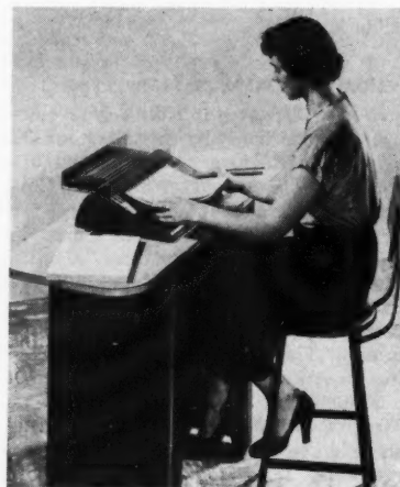
Model GB binder, with companion punch (not shown), are plastic binding equipment made by General Binding Corporation of Chicago
